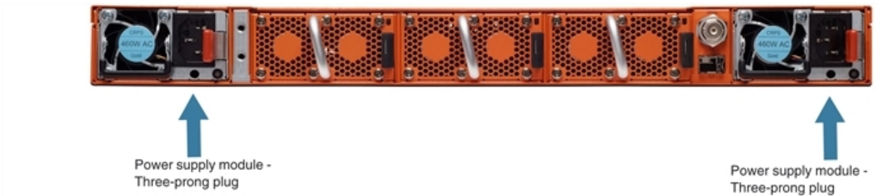
Figure 2 Connecting AC Power (GigaVUE-HCI)
