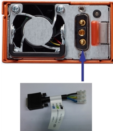
Figure 4 Connecting DC Power Supply Module
